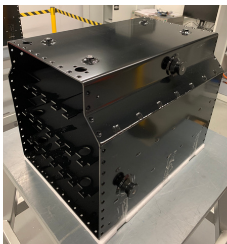
3. insulating worktable with the housing of a battery pack.
