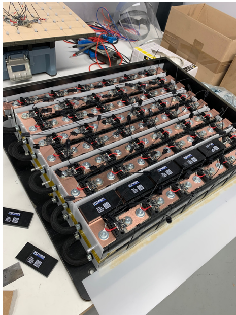
2. Rows of modules with the synthetic plates on the side. The top will be covered.
